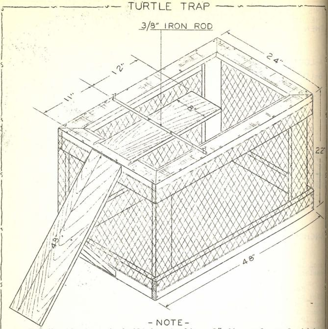
This turtle trap is built by stapling 1" diagonal mesh chicken netting on the bottom and sides of a frame work of 4" boards. A 6" strip of tin or galvanized iron is tacked around the top edge and bent down inside the trap. This prevents the turtles from crawling out of the trap.
