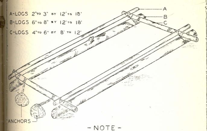
Green logs and brush are more desirable than dry because green wood lasts longer under water than dry wood, however, use the kind easiest to secure.
